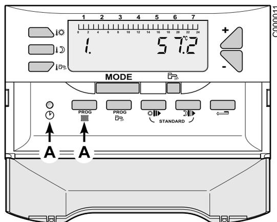
A=Access to the level fitter by simultaneous support during 5 seconds
